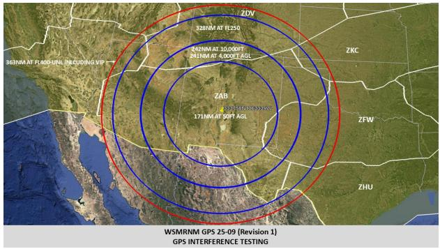
WSMRNM GPS 25-09 (REVISION 1) GPS INTERFERENCE TESTING
