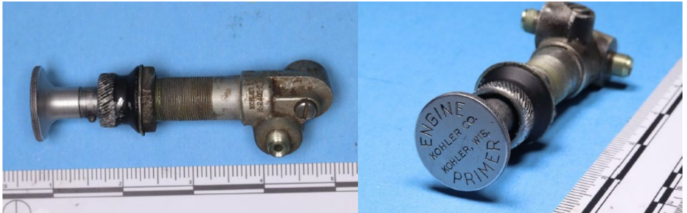
Fuel primer pump as received after the accident.
