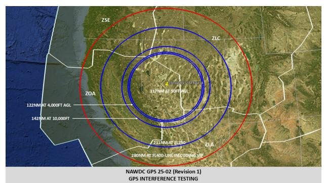
NAWDC GPS 25-02 (REVISION 1) GPS INTERFERENCE TESTING
