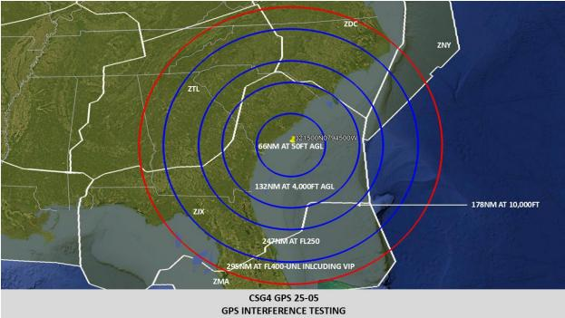
CSG4 GPS 25-05 GPS INTERFERENCE TESTING
