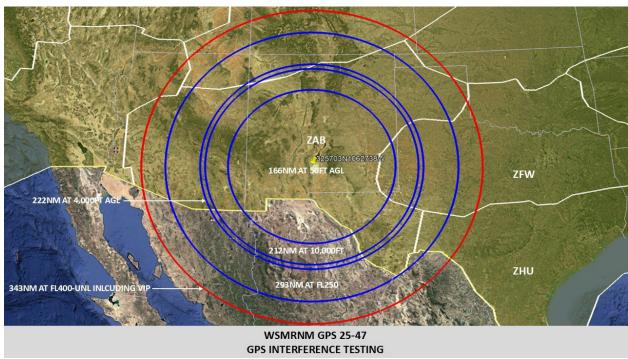
WSMRNM GPS 25-47 GPS INTERFERENCE TESTING
