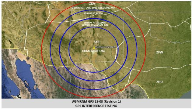
WSMRNM GPS 25-08 (REVISION 1) GPS INTERFERENCE TESTING
