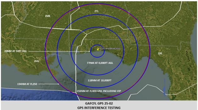
GAFCFL GPS 25-02 GPS INTERFERENCE TESTING
