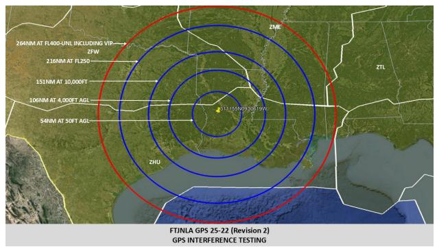
FTJNLA GPS 25-22 (REVISION 2) GPS INTERFERENCE TESTING
