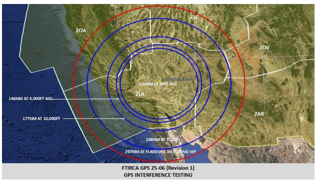
FTIRCA GPS 25-06 (REVISION 1) GPS INTERFERENCE TESTING
