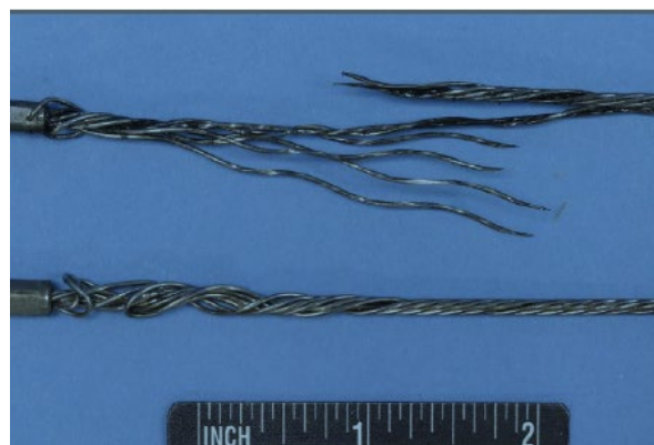
Figure 1. Worn throttle cables in need of replacement.
