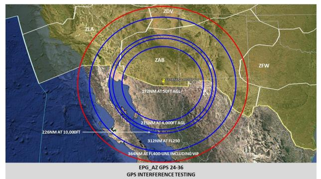
EPG\_AZ GPS 24-36 GPS INTERFERENCE TESTING
