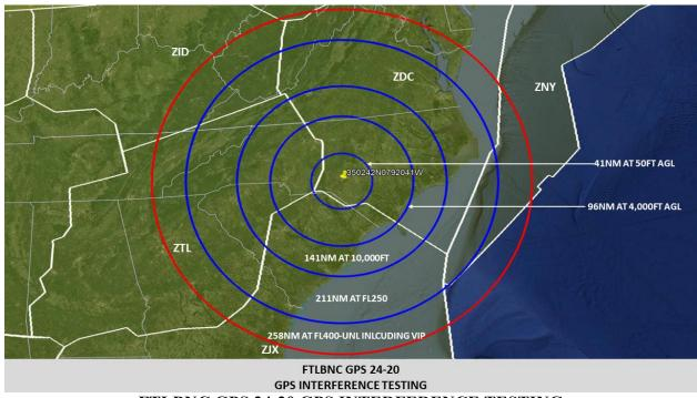
FTLBNC GPS 24-20 GPS INTERFERENCE TESTING
