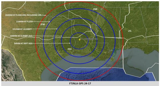
GPS INTERFERENCE TESTING FTJNLA GPS 24-17 GPS INTERFERENCE TESTING
