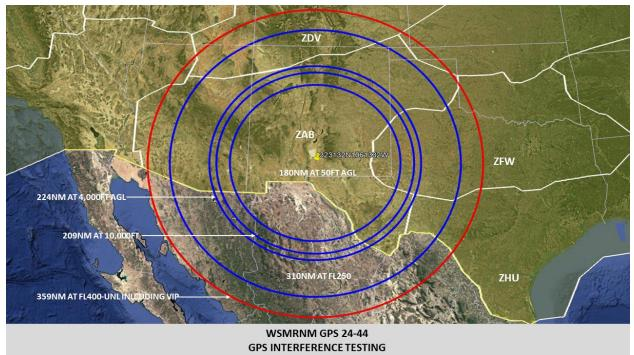
WSMRNM GPS 24-44 GPS INTERFERENCE TESTING
