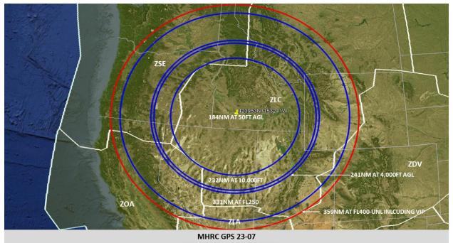
GPS INTERFERENCE TESTING MHRC GPS 23-07 GPS INTERFERENCE TESTING
