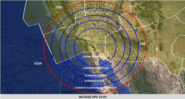
GPS INTERFERENCE TESTING MCASAZ GPS 23-03 GPS INTERFERENCE TESTING
