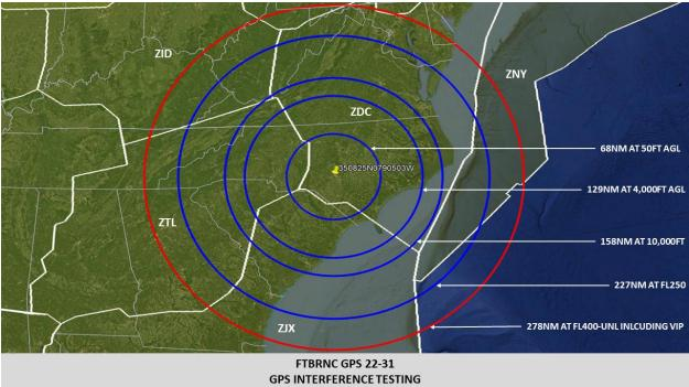
FTBRNC GPS 22-31 GPS INTERFERENCE TESTING
