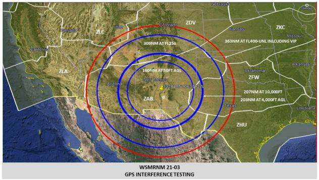
WSMRNM 21-03 GPS INTERFERENCE TESTING
