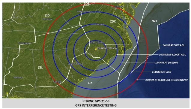
FTBRNC GPS 21-53 GPS INTERFERENCE TESTING
