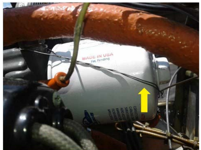
This oil filter was not properly safety wired. The wire is routed in the right direction, but there are too few twists per inch. The arrow points to the section with no twist.
