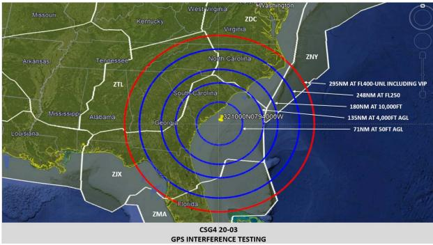
CSG4 20-03 GPS INTERFERENCE TESTING
