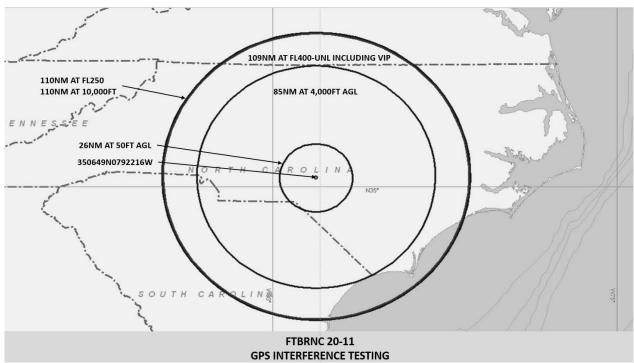
FTBRNC 20-11 GPS INTERFERENCE TESTING
