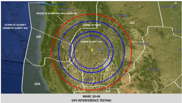
MHRC 20-04 GPS INTERFERENCE TESTING
