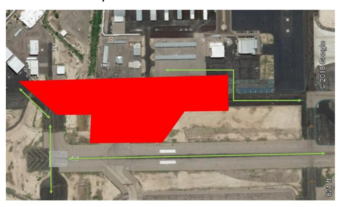
Phase 1C – 14 Days Runway 3/21 restricted to Group 2 aircraft (wingspan 79 feet or less). Runway 3/21 not usable for Air Carrier or F-16 arrival or departures. Portions of Delta and Delta 1 are closed. Old Delta 2 is decommissioned. New Delta 2 is open.
