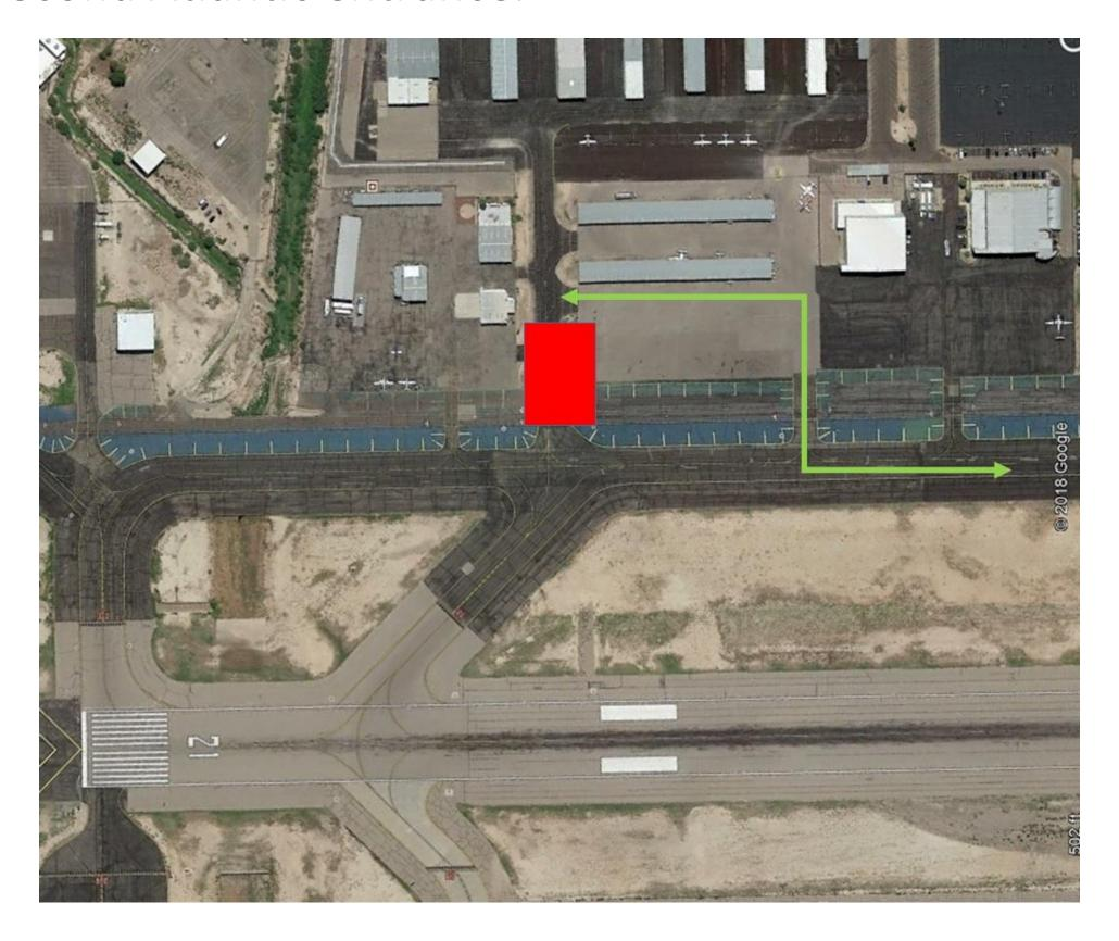
Phase 1B – 70 Days Runway 3/21 restricted to Group 2 aircraft (wingspan 79 feet or less). Runway 3/21 not usable for Air Carrier or F-16 arrivals or departures. Portions of Delta north of Alpha is closed. Runway 21 PAPI and REIL out of service for 10 days.
