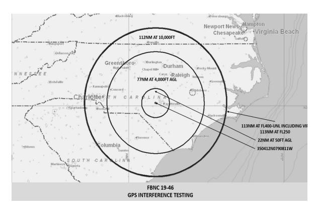
FBNC 19-46 GPS INTERFERENCE TESTING
