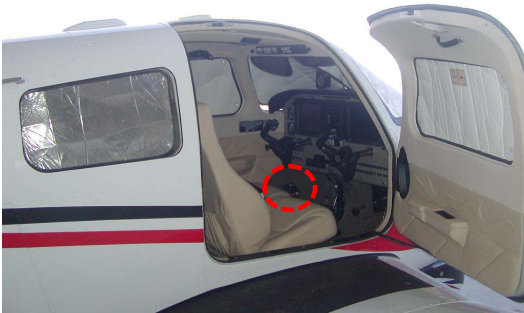
Figure 3: PA-28 Cockpit View Showing location of Generation 3 Fuel Selector
