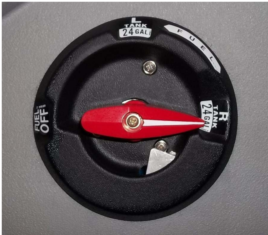
Figure 4: Generation 3 Fuel Selector (Preferred fuel selector)
