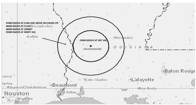
FTPK 18-39L GPS INTERFERENCE TESTING
