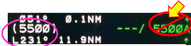
Figure 1a. “Climb to” 5500 feet then Left turn to 231° Course to Fix. (Fix is not shown.)
