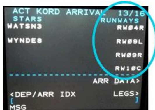
Figure 5b. ARRIVALS page selections for Runway extension in FMS 4.x (Types 7 and 8 Navigation databases)
