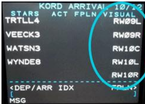
Figure 5a. ARRIVALS page selections for Runway extension in FMS 3.x (Type 6 Navigation databases)
