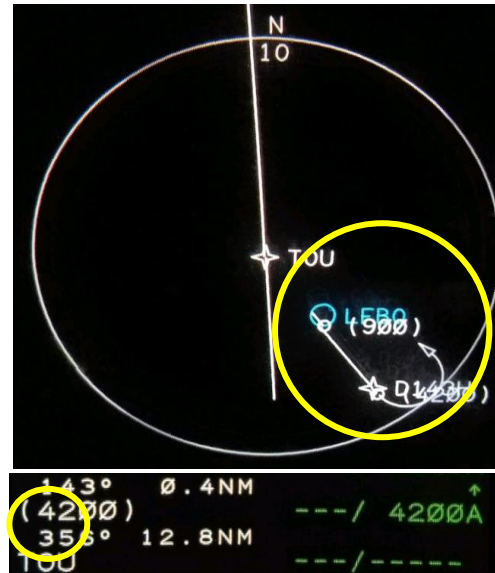
Figure 3b. After manually entering 4200A (in places of 4000A), the "R" turn direction is removed and the FMS computes the shortest turn direction, left in this case.
