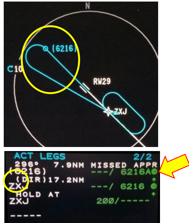
Figure 2b. After the crew uses the left FMS to activate Temperature Compensation, the "R" turn to ZXJ is initially removed (blanked) on the right FMS and will subsequently be removed on both FMSs. The map display may differ from this example.
