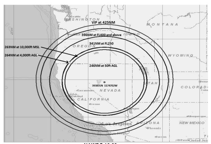
NAWDC 16-03 GPS INTERFERENCE TEST
