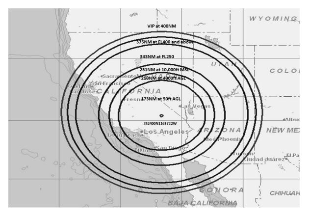
**NTC 15-03 GPS INTERFERENCE TESTING**
