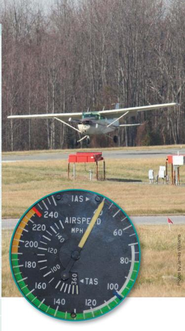
As you know (and as shown in the chart),  $V_A$ is one example, because the numerical value of  $V_A$ changes with weight. Another example concerns  $V_X$ and  $V_Y$ : as altitude increases,  $V_X$  increases slightly and  $V_Y$  decreases.  $V_X$  and  $V_Y$  are equal when the airplane reaches its absolute ceiling.
