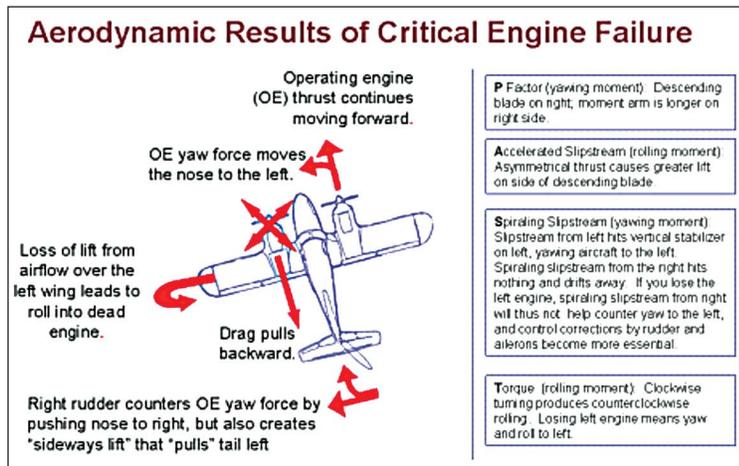
The yaw and roll forces must be counteracted by a combination of rudder and aileron.
