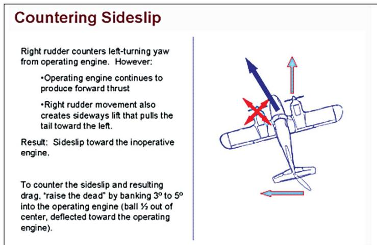
Sideslip is the angle at which the relative wind meets the longitudinal axis of the airplane. In all-engine flight with symmetrical power, zero sideslip occurs with the ball of the slip-skid indicator centered. Pilots know this concept as "coordinated flight." In OEI flight, however, zero sideslip occurs with the ball slightly out of center, deflected toward the operating engine.
