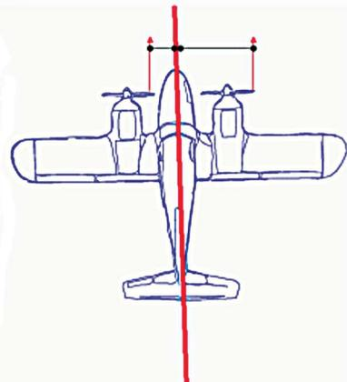
Some twins of more recent design use a counter-rotating right engine to eliminate the critical engine. Handling qualities are the same, regardless of which engine fails on one of these airplanes.
