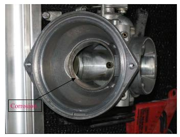
Corrosion was also observed on the carb slide itself (sometimes called piston) as well as some buildup of a varnish like substance.
