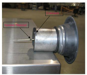
Inspection of the slide revealed significant build ups of corrosion on the slide. The corrosion was especially thick on the bottom edge of the slide.
