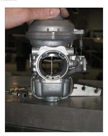
In a normally operating Bing carburetor the slide would always be pushed down to the bottom of the carb body by a combination of gravity and pressure from a compression spring in the carb dome that pushes down on the slide itself.
