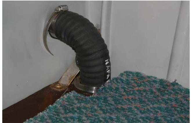
We found, among other things, that the installer used an automotive radiator hose and clamps for the filler. Additionally, the installer failed to change the baggage weight placard that would have been part of the STC
