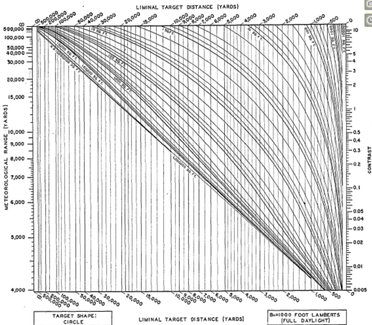
Figure 11. Nomogram showing threshold target distance as a function of target area, Weber contrast ratio, and meteorological range of the atmosphere. From Duntley (1948).
