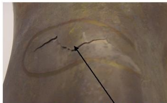
Crack through aft side of tailpipe
