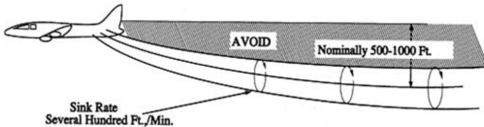
**Wake turbulence blows** with the prevailing wind, which can take it away from runways if there’s a crosswind, but can cause it to interfere with operations on an intersecting or parallel runway. Wake turbulence generated by helicopters operating in ground effect can be extremely intense, similar in theory to a microburst, and follow a similar drift pattern.
