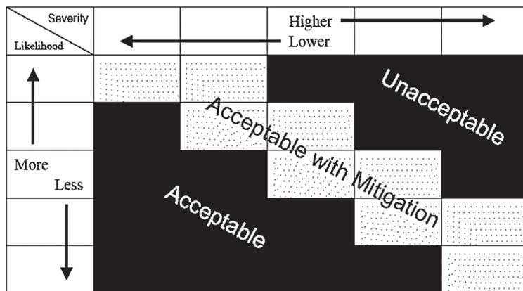
Assessment of risk is an important part of good ADM. The hazard described above—a nick in the propeller—poses a risk only if the airplane is flown. If the damaged prop is exposed to the constant vibration of normal engine operation, there is a high risk is that it could fracture and cause catastrophic damage to the engine and/or airframe (not to mention the occupants of the aircraft!).
