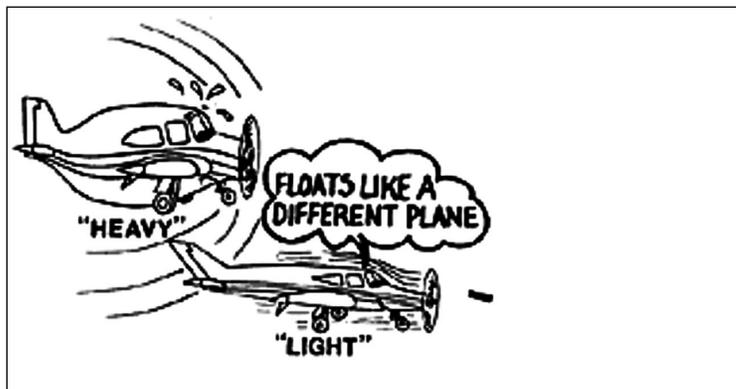
Remember, the 1.3  $V_{so}$  formula is based on the actual weight of the aircraft, not the maximum landing weight. If you use your customary maximum weight 1.3  $V_{so}$  number all the time, the aircraft will float as it dissipates the excess energy. Assuming that you will want to land at or close to the stall speed, runway distance will be eaten up during the process.
