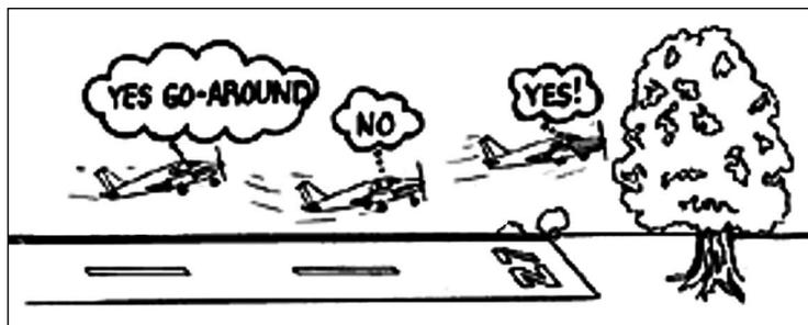
Treat the go-around as a normal procedure, not an abnormal or emergency action. Always be prepared to go around. Experienced pilots always determine in advance a go-around point on the runway. If they have not touched down by that point, it is go-around time.
