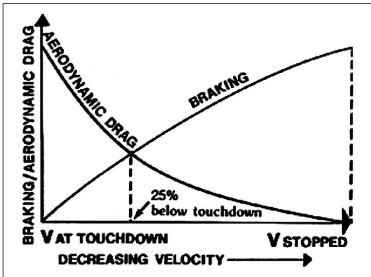
Apply brakes after all three wheels are on the runway and the airplane has slowed to at least 25 percent below touchdown speed. In fact, for most airplanes, aerodynamic drag is the single biggest factor in slowing the aircraft in the first quarter of its speed decay. Brakes become increasingly effective as airspeed and lift decrease.
