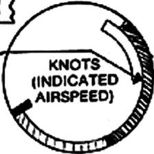
If you use CAS as  $V_{so}$ , however,  $1.3 \times 50 = 65$  knots CAS. Referring to the correction table, the IAS for an approach (at maximum landing weight in smooth air) would be 63 knots IAS, given an actual safety margin of 15 knots above the real, or calibrated, stall airspeed. The safety margin, however, will look like a margin of 23 knots on your airspeed indicator.
