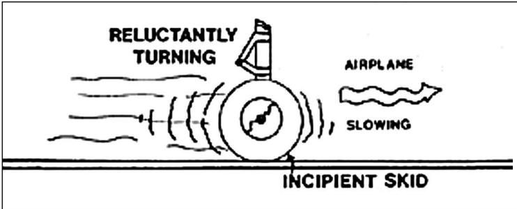
Whatever you do, don't lock the wheels. Braking effectiveness drops dramatically in a skid, and tires could be damaged.
