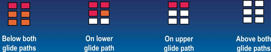
Three Bar VASI installations provide two visual glide paths. The higher glide path is intended for use only by high cockpit aircraft (Boeing 747, DC10) to provide a sufficient threshold crossing height.
