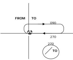
If lateral spacing is proper, needle will be "dead" on the side of the case when the inbound turn begins. Needle should begin to move within 45 degrees of inbound course. If no movement, stop inbound turn at 45 angle and wait until needle begins to move. If needle leaves side of case before 45 degree point, continue standard rate turn and then correct into the needle.
