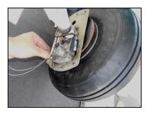
Starting on the top bolt, safety wire with positive tension, then wrap around the bottom bolt.
