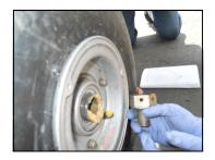
Some of the grease will come out of the bearings, just wipe it off with a rag.
