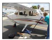
· Slide wheel assembly onto axle
