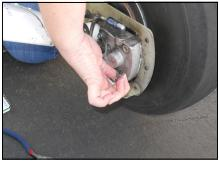
Slide brake pad out from behind the brake caliper
