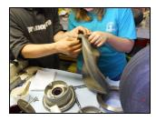
Coat new tire and tube with talc powder
