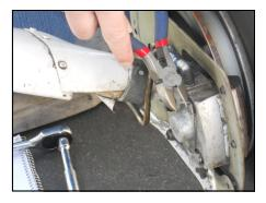
Snip the safety wire holding the brake pad on.
