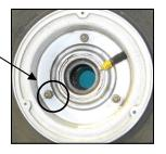
For the best leverage, hold backside of bolt with wrench while using ratchet on nut.
