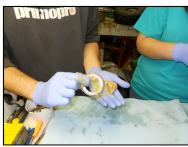
Push the grease into one section and continue until the grease pushes through to the other side. Rotate the bearings until full of grease.
