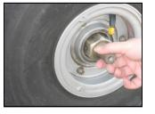
Wheel should slide off of the axle easily
