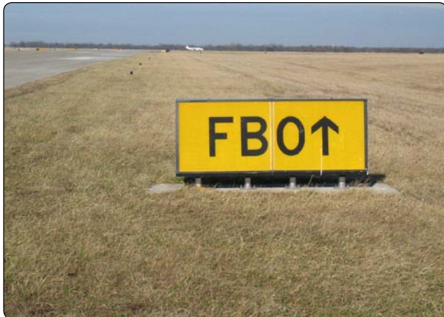
Figure 1-34. Destination sign to the fixed-base operator (FBO).
