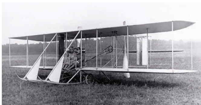
The Wright Flyer Model B paved the way for the conventional style empennage we see in most aircraft today.
