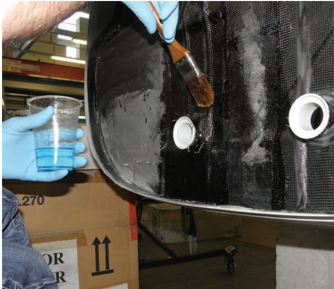
Applying resin to a woven fabric style of reinforcement is one common method of creating a composite material.
