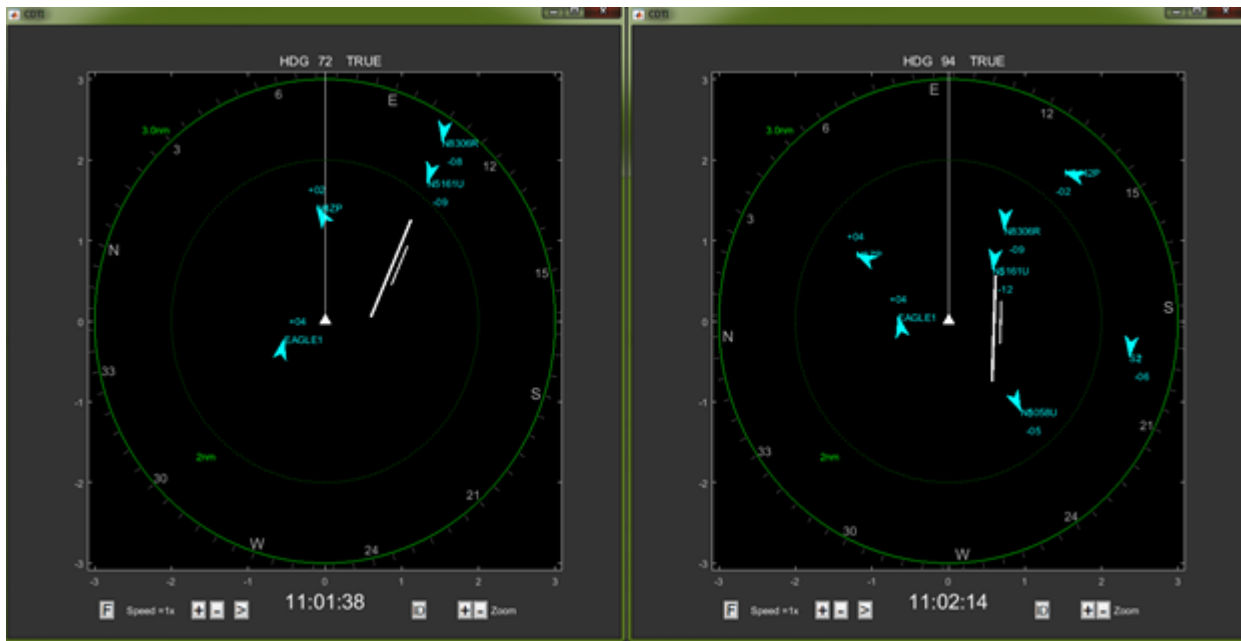
Figure 12. Simulated in-cockpit traffic display for N1285U at 1101:38 (left) and 1102:14 (right).
