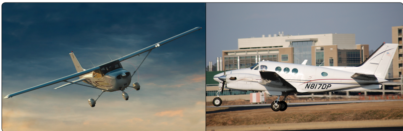
Figure 7-39. Fixed (left) and retractable (right) gear airplanes.
