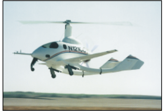
Figure 15-3. The CarterCopter uses wings to enhance performance.
