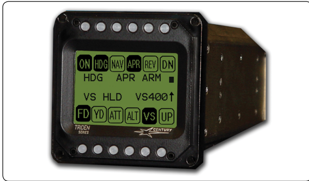
Figure 2-23. An example of an autopilot system.
