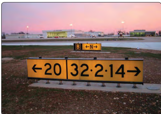
Figure 14-23. Runway destination sign with different taxi routes.
