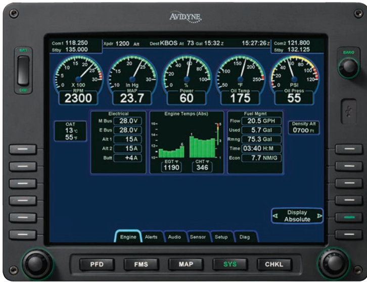
This MFD screen shows information from an engine monitoring device.
