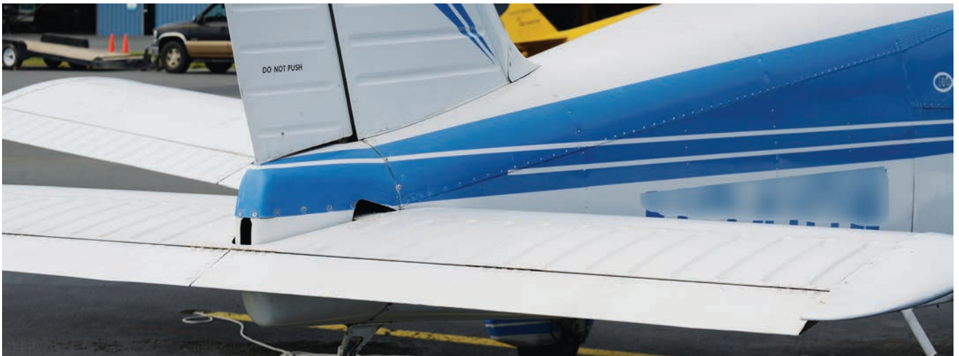
Autopilots make use of trim tabs to help control the airplane.
